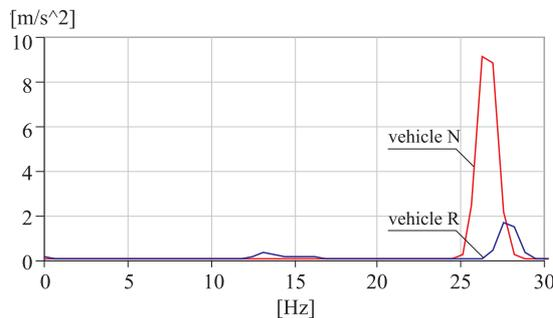
Fig. 4. Signal spectrum for measuring point 5 at the speed of 70 km/h; main components: vehicle N – 26.25 Hz, 9.2 m/s<sup>2</sup>, vehicle R – 27.50 Hz, 1.6 m/s<sup>2</sup> [own study]
