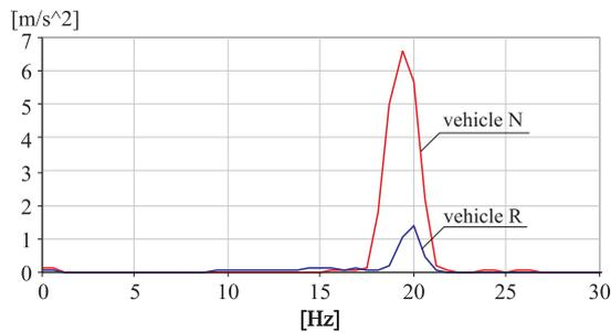
Fig. 3. Signal spectrum for the 6Y measurement point at 40 km/h; main components: vehicle N – 19.38 Hz, 6.6 m/s<sup>2</sup>, vehicle R – 20.00 Hz, 1.4 m/s<sup>2</sup> [own study]
