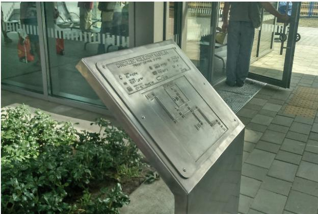
Fig. 4. Tactile graphics at the station in Nasielsk [14]
