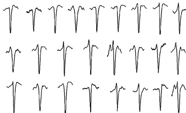
Fig. 1. 25 (from 50) real signals from transverse cracks that was used for ANN training
