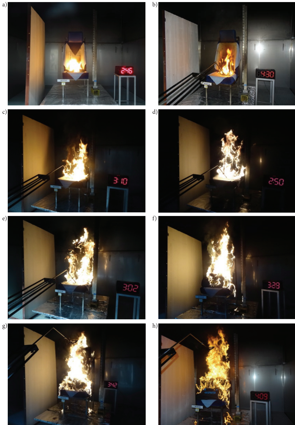
Fig. 5. Tests with different types of ignition sources. Seats ignited by: a) paper cushion (according to UIC 564-2 and PN-K-02502:1992), b) gas burner 7 kW, c) gas burner 15 kW, d) gas burner 25 kW, e) gas burner 50 kW, f) small travel bag ignited by paper cushion, g) travel bag ignited by gas burner of 25 kW/90 s, h) 2 travel bags ignited by gas burner of 25 kW/90 s. [source: Archives of Laboratory]
