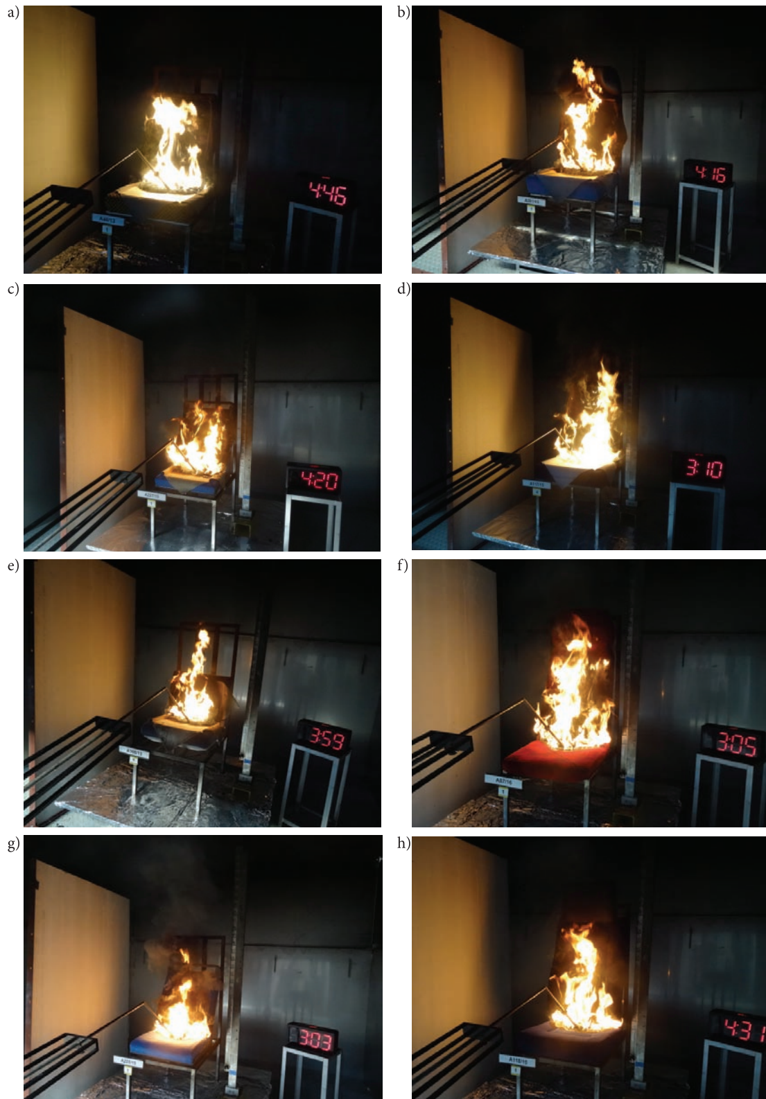
Fig. 2. Different types of passenger seats tested according to new proposal of EN standard: a) seat No A46/13, b) seat No A381/13, c) seat No A227/15, d) seat No A117/15, e) seat No 366/13, f) seat No A87/16, g) seat No A228/15, h) seat No A118/15 [Source: Archives of Laboratory]
