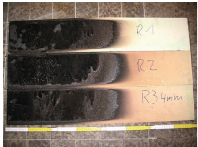
Fig. 8. GFK grey inside CFE = 22 kW/m 2
