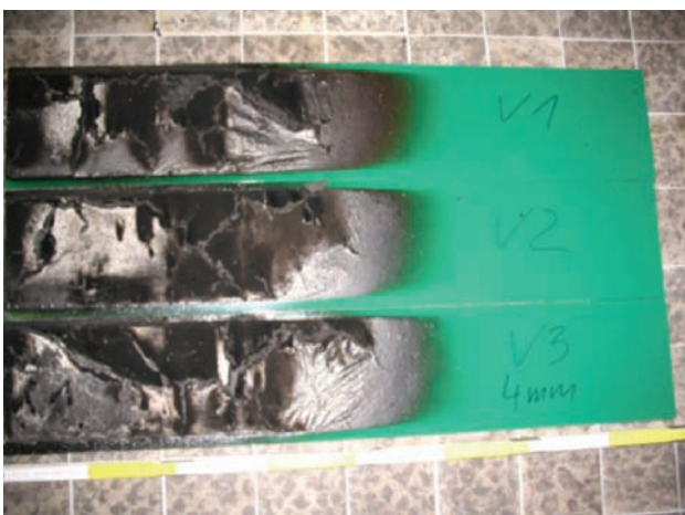
Fig. 7. GFK green outside CFE = 22 kW/m 2
