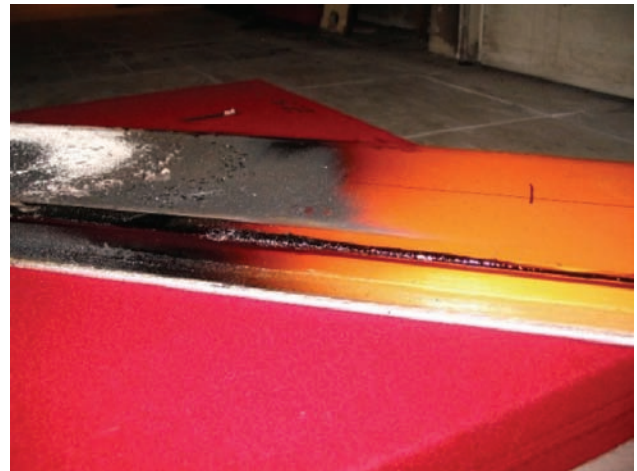
Fig. 20. Test material for the cone test: a) with honeycomb structure: b) and for spread of flame test closed structure
