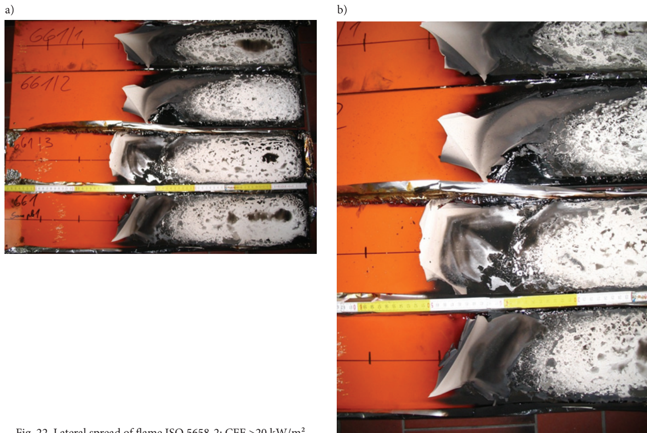
Fig. 22. Lateral spread of flame ISO 5658-2; CFE >20 kW/m 2
