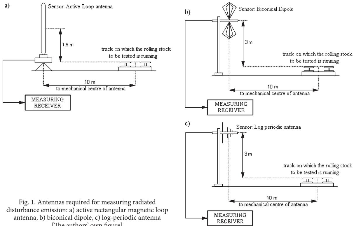
Fig. 1. Antennas required for measuring radiated disturbance emission: a) active rectangular magnetic loop antenna, b) biconical dipole, c) log-periodic antenna [The authors' own figure]
