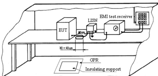
Fig. 1. General test-bench for laboratory research
