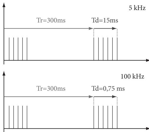
Fig. 6. BURST of disturbance impulse parameters for  $f = 5 \text{ kHz}$  and  $100 \text{ kHz}$  [Own figure]
