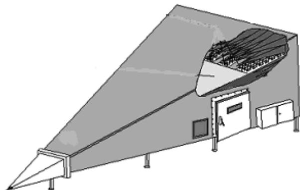
Fig. 2. The GTEM chamber [Own figure]
