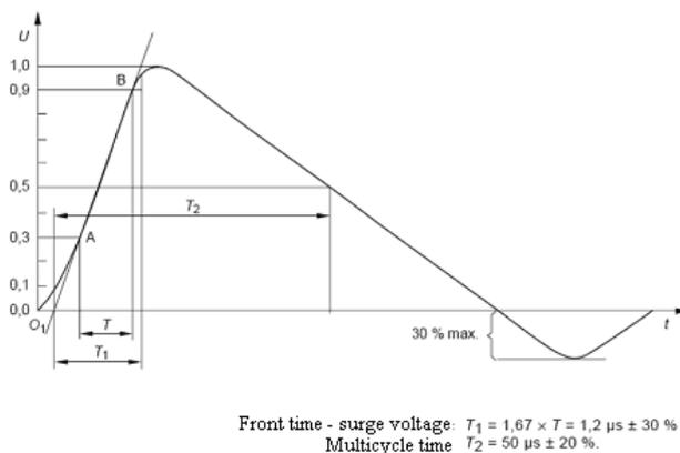
Fig. 3. The parameters and shape of the surge impulse
