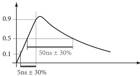
Fig. 5. The graph BURST 5/50 ns impulses [Own figure]
