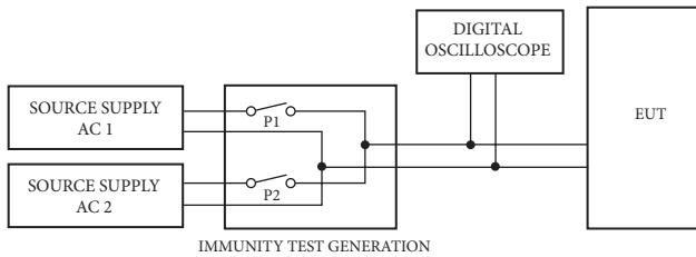
Fig. 8. The block diagram of measurement system
