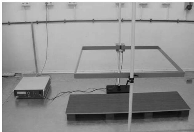
Fig. 10. The test-bench for research of resistance to pulsed magnetic field [Institute's own pictures]
