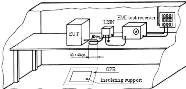
Fig. 1. General test-bench for laboratory research
