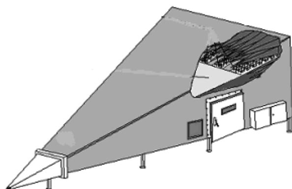
Fig. 2. The GTEM chamber [Own figure]
