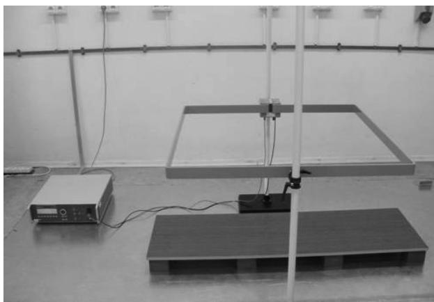
Fig. 10. The test-bench for research of resistance to pulsed magnetic filed [Institute's own pictures]
