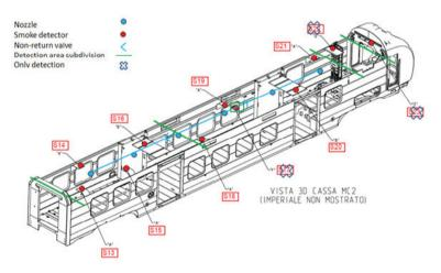
Fig. 7. Layout of a fire detection and firefighting system for passenger areas for the vehicle object of our example. This layout is subject to design validation via smoke tests and full scale fire tests
