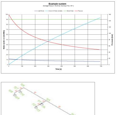
Fig. 8. Calculation of stored water quantity for the passenger areas
