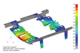
Fig. 6. FEM calculation of frame for high pressure water mist cylinders
