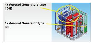
Fig. 5. Example of the position of aerosol generators
