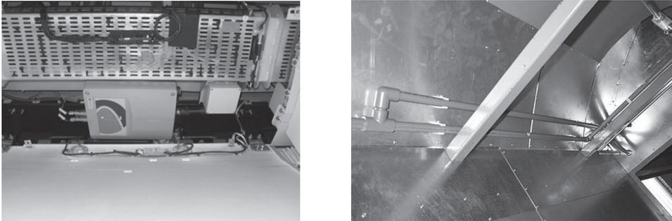
Fig. 7. Example of integration in the carbody of a smoke aspiration system
