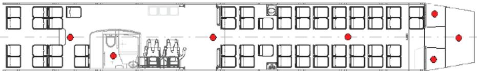
Fig. 6. Example of possible positions of point smoke detectors in a EMU driving coach. Can be seen three detectors in passenger areas, one in the toilet, one in the driving cab and two protecting the medium voltage electrical cabinets placed right behind the driving cabin
