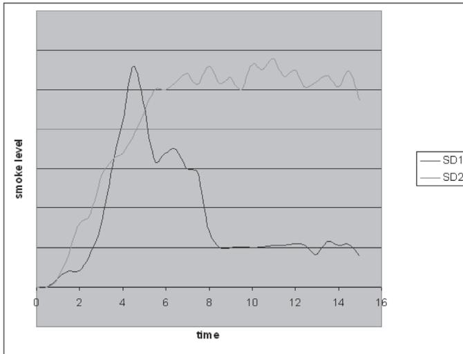
Fig. 3. Smoke level threshold value (red line), confirmed fire alarm (SD2), exceeded threshold for a certain time, or aborted when smoke value lower down again (SD1)
