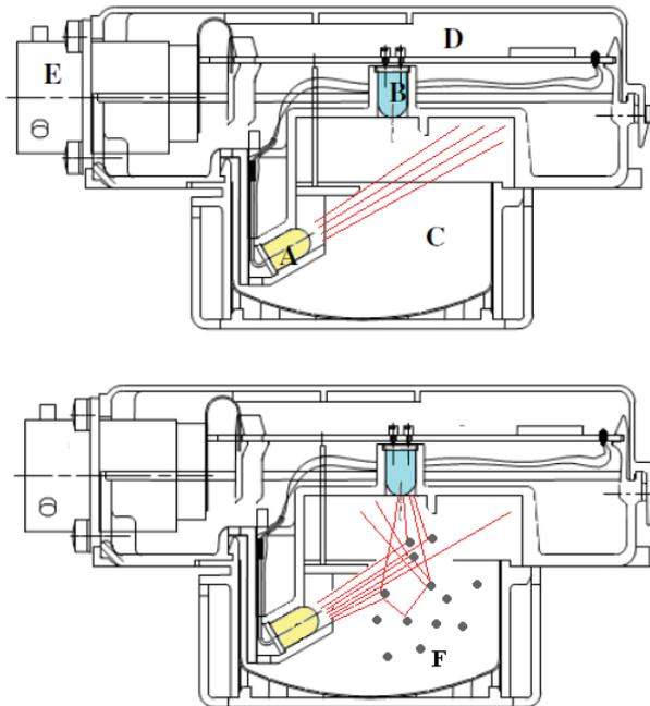
Fig. 1. Internal components of a smoke detector and scattered light principle:
