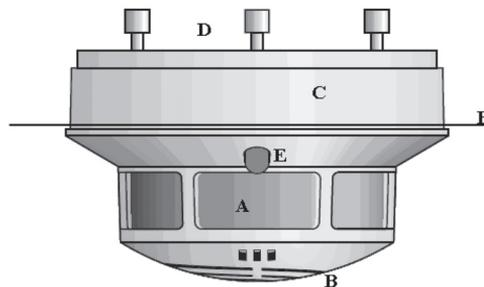
Fig. 2. General layout of a smoke detector: A) measuring chamber, B) housing with openings for smoke entrance, C) housing for motherboard and electrical connectors, D) electrical connectors, E) external LED for status information, F) line of the ceiling, indicating the hidden and on view parts
