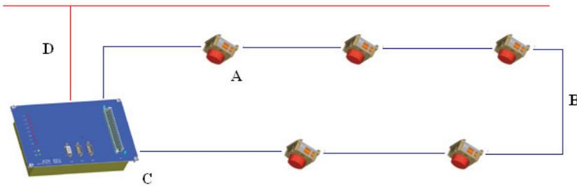
Fig. 4. Example layout of smoke detection system, based on point smoke detectors connected in loop with a central processing unit: A) point smoke detectors, B) connecting loop, C) central processing unit, D) communication with train control management system
