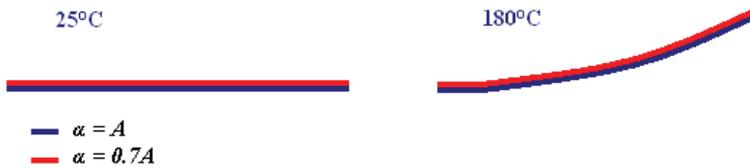
Fig. 12. A sheet made by two materials coupled, having different thermal expansion coefficient, will bend in the direction of the material having the lower coefficient, when subjected to a temperature increase
