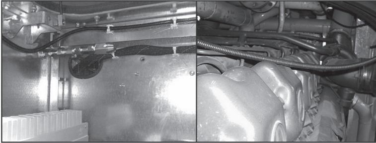
Fig. 10. Example of LHD cable and protective wire installation, along the internal walls of an electrical box (left, also fixing fasteners can be seen) or lying over cylinder head and turbocharger of a diesel locomotive engine (right)
