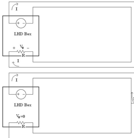
Fig. 9. Linear heat sensitive electrical detector layout. If the wires are melted, the line is short-circuited and the voltage at monitoring resistor  $R$  is zero
