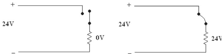
Fig. 13. Example of basic circuit with an integrated thermal switch. Depending on the design, several additional components (resistors, ammeters etc.) can be present; the switch can be normally closed or normally open
