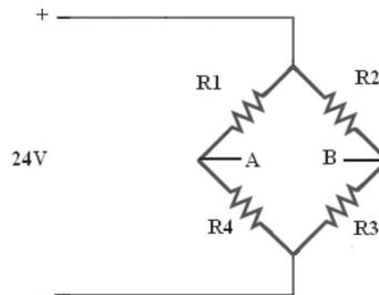
Fig. 11. Wheatstone bridge for resistance thermometer
